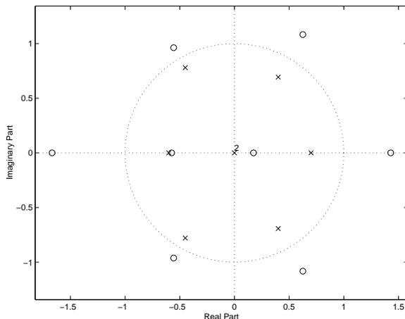
Fig. 4: Pole-zero plot upon convergence of the adaptive system estimator for example system 1, with  $N = 8$  and  $M = 6$ .
