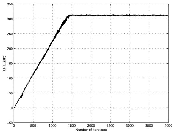
Fig. 2: Convergence characteristic of the adaptive algorithm for example system 1 ( $\mu = 0.07$ )
