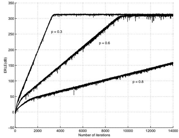
Fig. 6: Convergence characteristic of the adaptive algorithm for the case of a coloured input signal ( $\mu = 0.04, 0.02$  and  $0.008$  for the cases  $p = 0.3, 0.6$  and  $0.8$  respectively)
