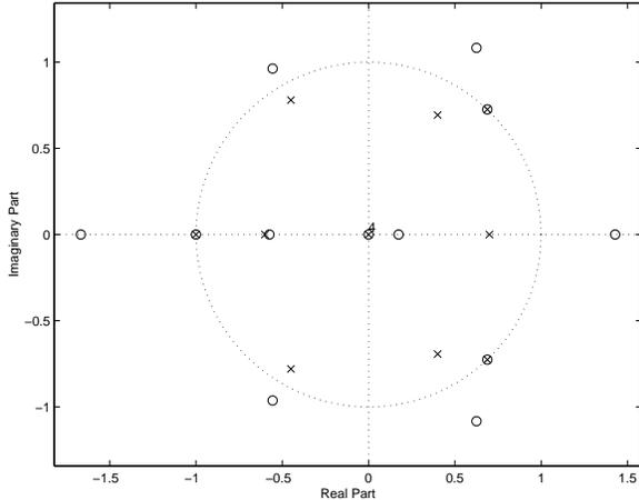
Fig. 5: Pole-zero plot upon convergence of the adaptive system estimator for example system 1, with  $N = 13$  and  $M = 9$ .
