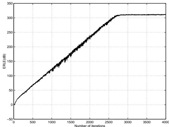
Fig. 3: Convergence characteristic of the adaptive algorithm for example system 2 ( $\mu = 0.05$ )
