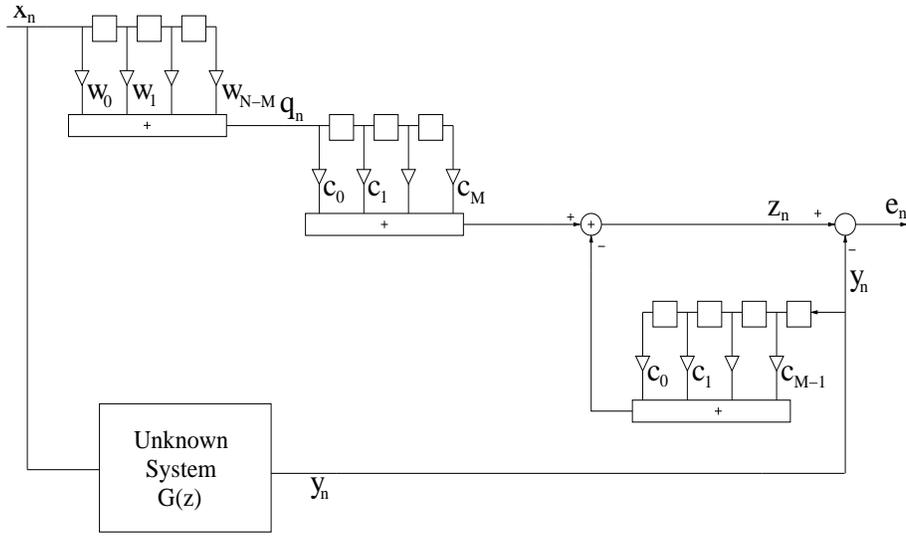
Fig. 1: Structure of the adaptive digital filter.
